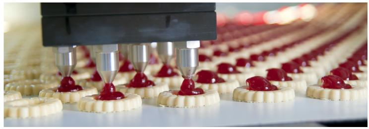
Pneumatics operate actuators and cylinders providing pick and place operations, as well as the dispensing of fillings, juices and fluids.
